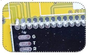
Ensure that all welding is in good condition, and there shall be no short-circuit and false welding. In the case of false welding in the figure below, the short-circuit position can be disconnected by soldering iron drag welding.
