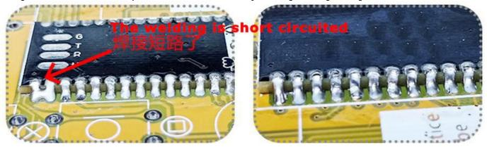
2. Welding USB power supply base: Note: USB needs to be installed correctly. It is installed according to the description of the silk screen symbol on the bottom plate. Several pins are empty and do not weld. At that time, because the pins are too close to prevent short circuit by welding, it is specially treated that three pads are not stained with tin and do not weld.
