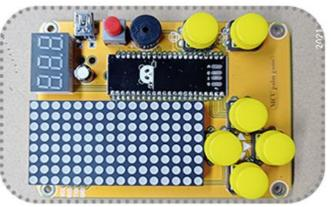
10. Power on test. Note: USB power supply and battery box power supply cannot be used at the same time, because USB power supply will cause the battery in the battery box to be charged, which may cause problems. In addition, the positive and negative poles of the battery box wiring shall be distinguished.
