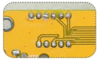
8. Welding dot matrix module. Note: the dot matrix module needs to be aligned in the direction, and there is an obvious Chinese prompt at the corresponding position on the circuit board. Align the prominent small point on the edge of the dot matrix module with the small window marked by the silk screen symbol on the PCB. When welding, two dot matrix modules can be welded to two welding points before fixing the dot matrix, then adjusting the alignment position and welding other solder ioints.
